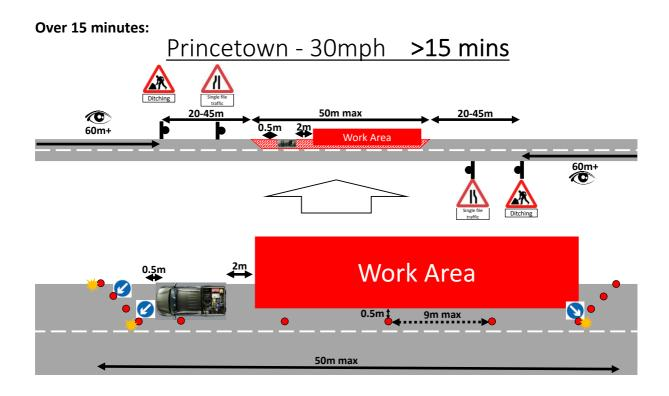
A4 – To minimise road traffic hazards, regulations require road signs and cones to be put in place in a specific order. This is shown below for the various layouts above.
